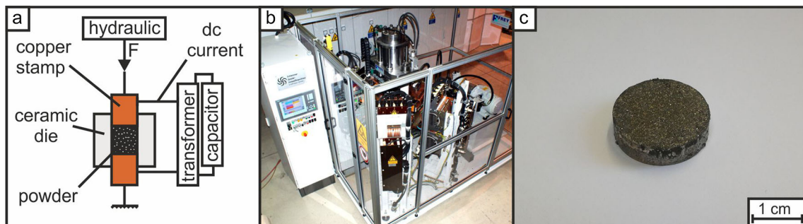
Fig. 2 a Schematic diagram of the principle of the EDS process and b the EDS machine of the Ruhr-University Bochum and c EDS-densified NdFeB magnet (diameter d = 19 mm)
