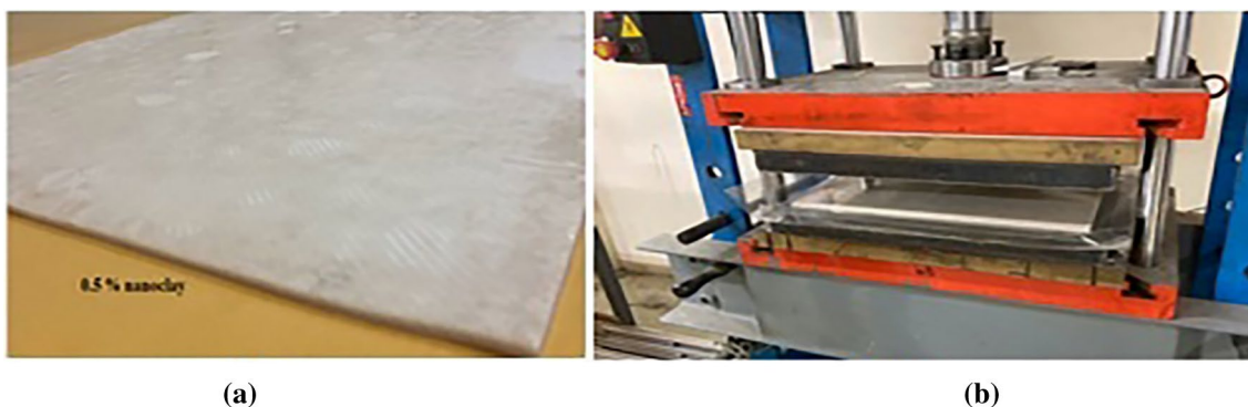
Figure 2 NC-reinforced glass fiber-reinforced composite plate manufacturing impregnated fabric.
