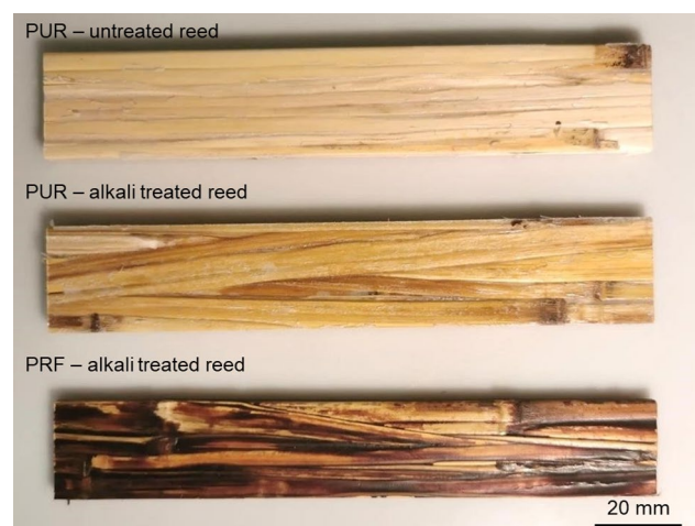
Figure 6 Optical appearance of different reed biocomposite beam specimens.
