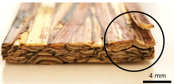
Figure 4 Spontaneous delamination of untreated reed stems bonded with phenol-resorcinol-formaldehyde resin after pressing.
