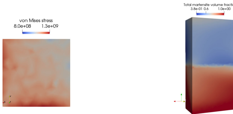
(e) Von Mises stress at a bi-crystal cross section parallel to x - y plane at \epsilon = 2\% (f) Corresponding total martensite volume fraction at \epsilon = 2\%
