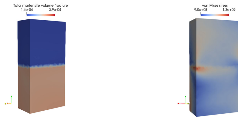
(c) Corresponding total martensite volume fraction at \epsilon = 0.3\% (d) Von Mises stress at a bi-crystal cross section parallel to x - z plane at \epsilon = 2\%
