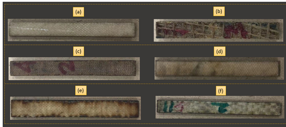
Figure 9 Composite samples from different woven fabrics developed in our laboratory: a flax woven fabric-reinforced PP composites, b jute woven fabric-reinforced MDI composites, c flax woven fabric-reinforced MDI nanocomposites (AgNP
