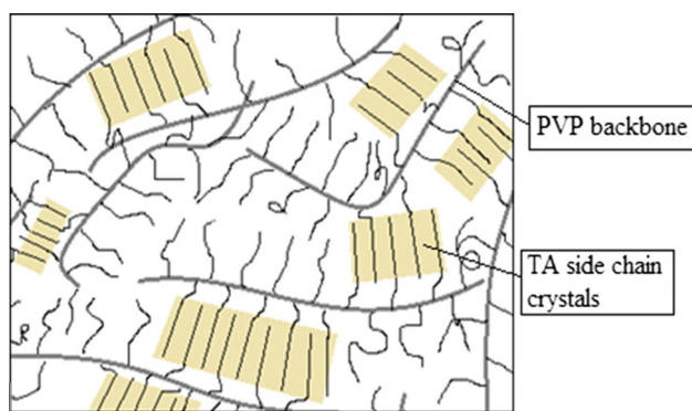
Figure 8 Schematic model for crystallisation of graft copolymers [37–39].
