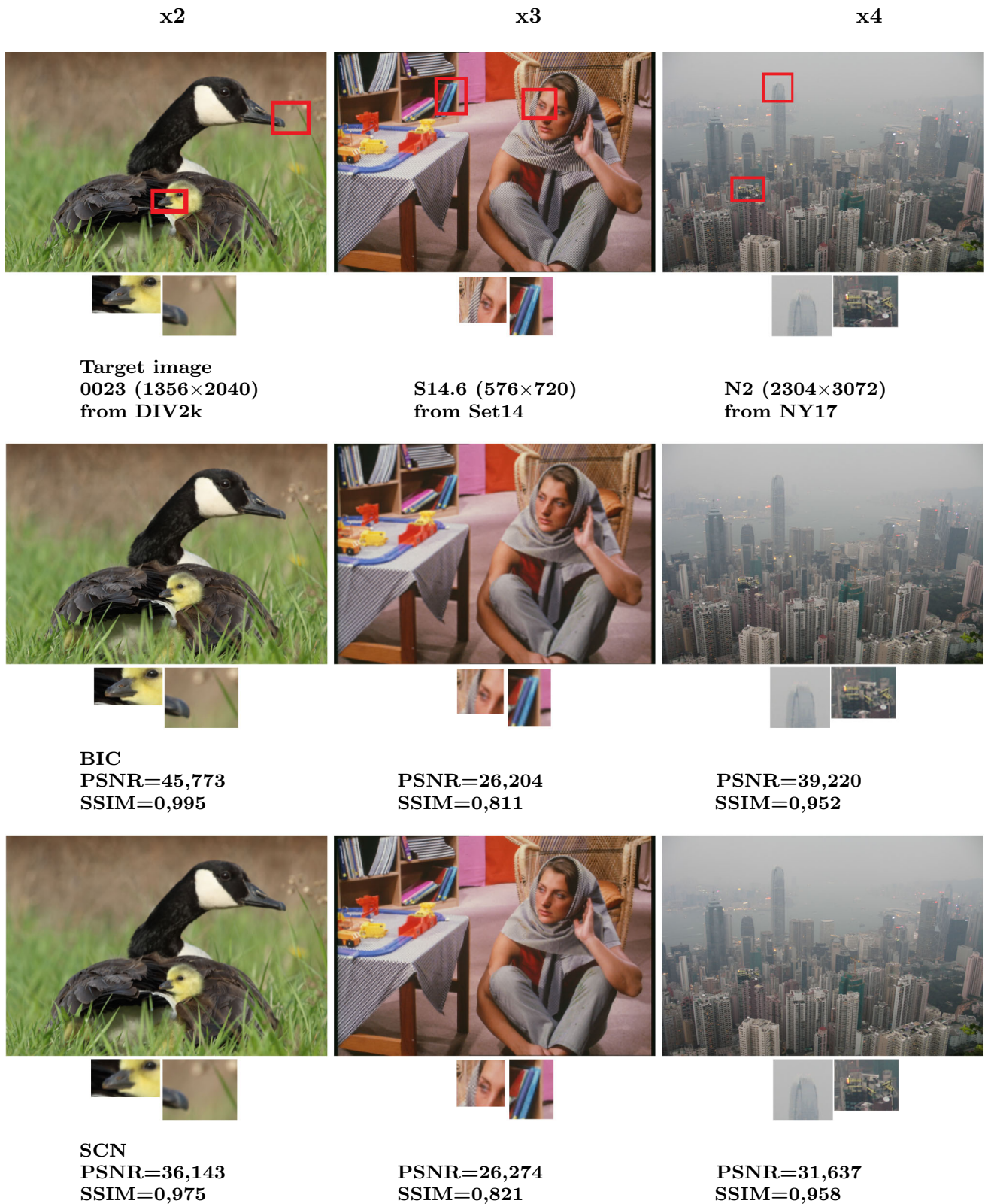
Fig. 7 Examples of supervised upscaling performance results at the scale factor 2 (left), at the scale factor 3 (middle), at the scale factor 4 (right)
