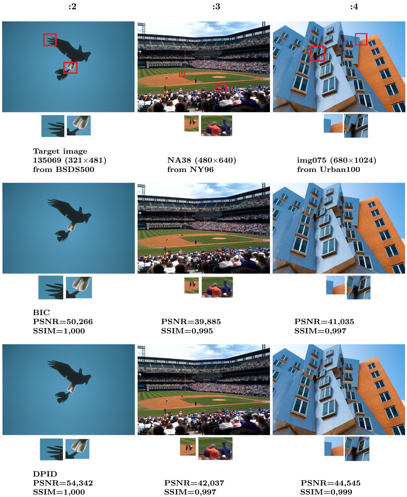
Fig. 9 Examples of supervised downscaling performance results at the scale factor 2 (left), at the scale factor 3 (middle), at the scale factor 4 (right)
