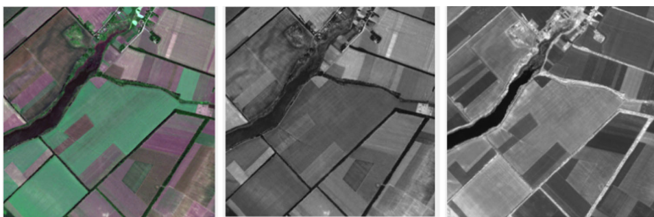
Fig. 1 Example. Left panel: the original noisy satellite image. Middle panel: its red channel. Right panel: near-infrared channel
