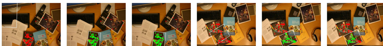
Fig. 12 Results from the two real registration experiment. From left to right: (3), (13), (2). Red means that the point was classified as outlier, green inlier. White frame shows registration of the model book under the estimated transformation (Color figure online)
