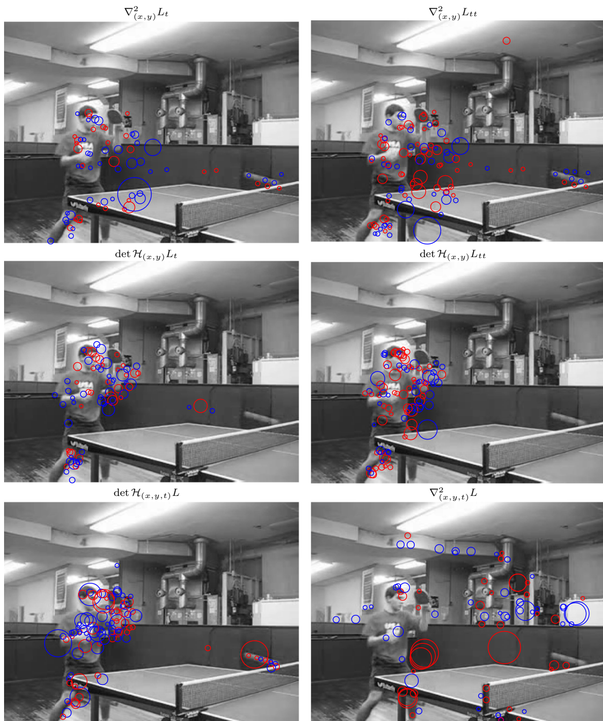
Fig. 8 Spatio-temporal interest points computed from a video sequence in the UCF-101 dataset (TableTennisShot_g10_c01.avi) for different scale-normalized spatio-temporal entities and using the presented time-causal and time-recursive spatio-temporal scale-space extrema detection algorithm with the temporal scale-space smoothing performed by a time-discrete approximation of the time-causal limit kernel for c = 2 and temporal scale calibration based on q = 1 : (Top left) The spatial Laplacian of the first-order temporal derivative \nabla_{(x,y)}^2 L_t . (Top right) The spatial Laplacian of the second-order temporal derivative \nabla_{(x,y)}^2 L_{tt} . (Middle row left) The determinant of the spatial
