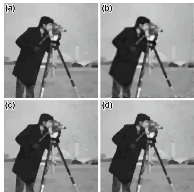
Fig. 14 Reconstruction of the cameraman-image corrupted by Gaussian white noise with \sigma = 0.1 and Gaussian blur. a pAPS (PSNR: 23.11; MSSIM: 0.7175), b SA-TV (PSNR: 22.64; MSSIM: 0.6957), c LATV (PSNR: 23.17; MSSIM: 0.7160), and d pLATV (PSNR: 23.15; MSSIM: 0.7160)
