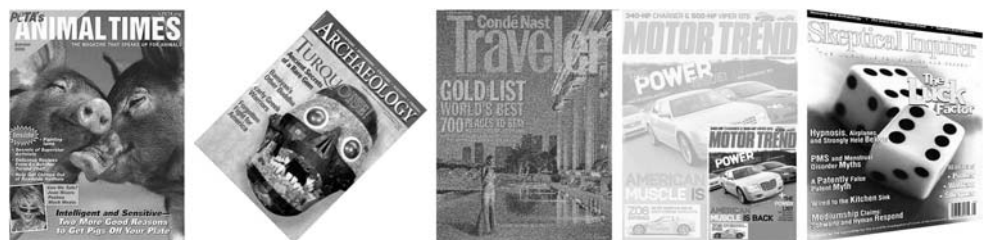
Fig. 1 A selection of data set images. From left to right: unchanged, rotated, added noise, scaled, changed perspective
