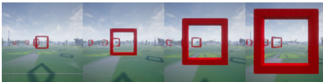
Fig. 2 Door views from various angles and orientations captured with the drone’s camera. The perception system determines the distance between the drone and the closest gate
