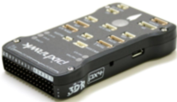
Fig. 4 Standard flight controller, Pixhawk ( https://commons.wikimedia.org/wiki/File:Pixhawk.png )
