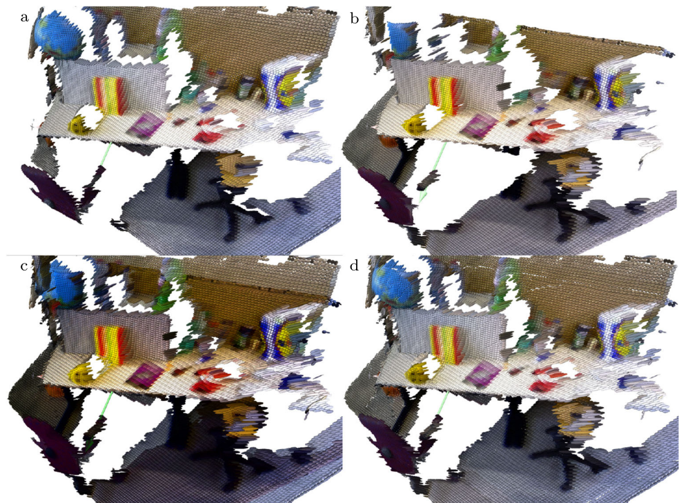
Fig. 7 Merging two local maps (a,b): maps in the common coordinate frame (c) and the obtained set of ellipsoids (d)
