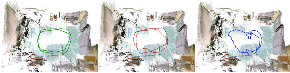
Fig. 16 Trajectories of the robot estimated by the ORB-SLAM2 during the experiment in the laboratory
