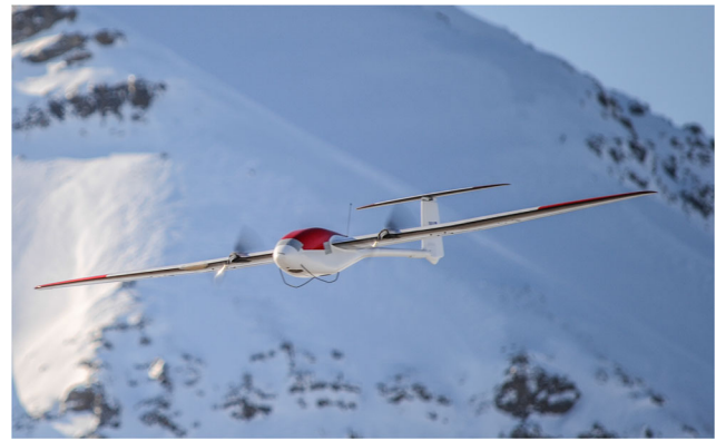
Fig. 2 The NTNU Cruiser-Mini fixed-wing UAV with cruise speed of approximately 20 m/s
