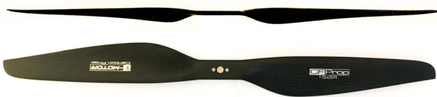
Fig. 3 T-Motor 15' × 5' propeller—Lateral and frontal view
