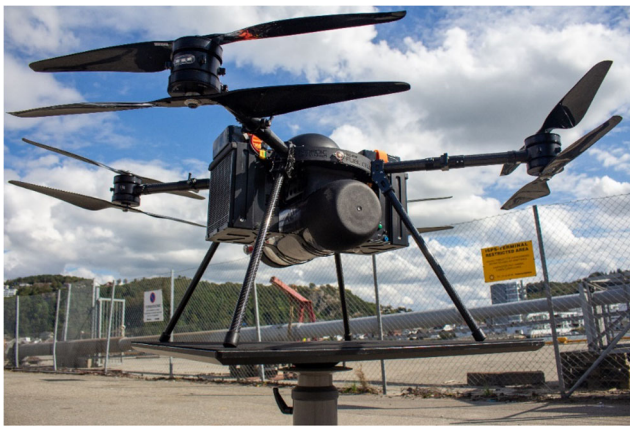
Fig. 2 Staker BG-200 FC from Nordic Unmanned with the reference fuel cell hybrid system installed
