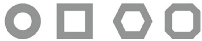
Fig. 2 Censure bi-level filters. From left to right: the ideal circle, octagon, hexagon and box. Image adapted from [1]
