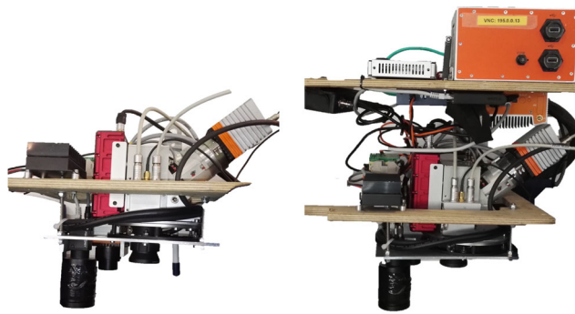
(a) Side view of the payload, (b) Side view of the full pay- with imaging sensors and IMU load.
