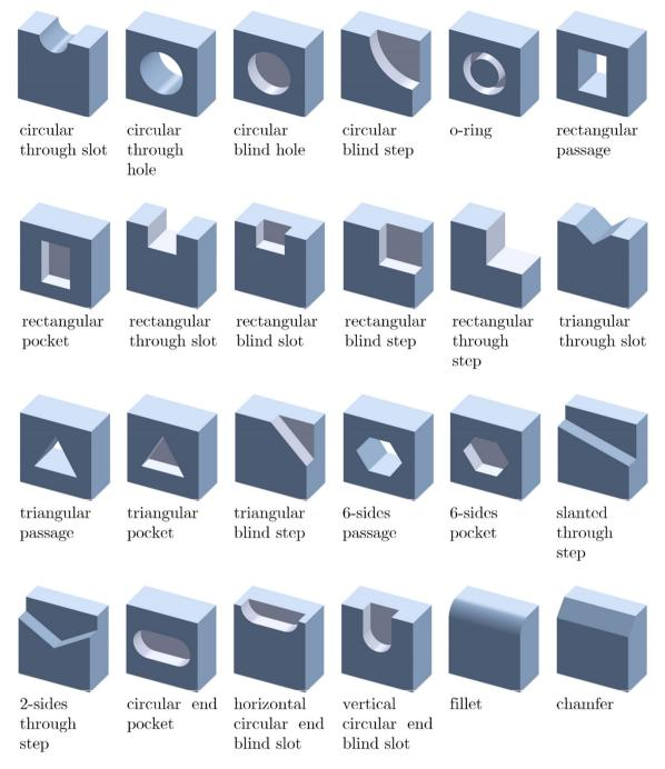
Fig. 6 Machining features present in the dataset, as suggested by Zhang et al. (2018)
