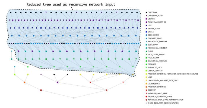
Fig. 1 Typical hierarchical structure representing the geometric data for a simple CAD model; connections show how low-level features are combined to form complex shape representations, the shaded region represents the portion of the tree which will be used as input for the neural network
