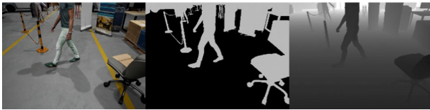
Fig. 4 Ground truth data output of UnrealCV used for training of SeS and DE model: RGB (left), object mask (center), depth (right)
