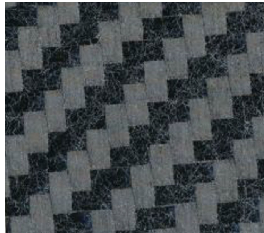
Fig. 3 The normal condition of the carbon fiber textile under study
