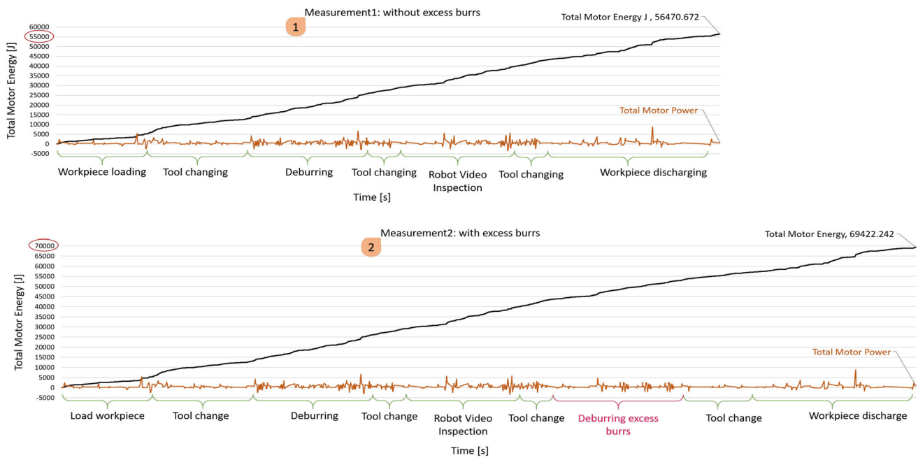
Fig. 9 Records of the total energy (marked in black) and total power (marked in orange) of the drive for the deburring process during a work cycle of a workpiece with no remaining burrs (1) and with remaining burrs (2)
