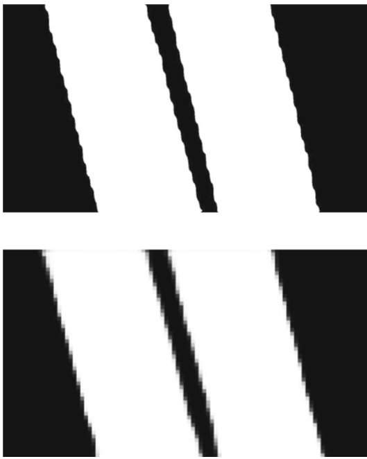
Fig. 15 The rescaling process of the segmentation masks causes irregular (image top) or blurred (image top) edges which has a great impact on the determination of the gap dimension. This occurs since the measurement accuracy is based on the number of pixels between the CFT edges. An anti-aliasing technique of the CFT edges could increase the accuracy of the inspection system. However, this approach goes beyond the scope of the present study. For comparison, one pixel has a size of approximately m_p = 0.0172 mm which is also the smallest measurable quantity
