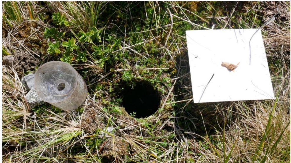
Fig. 2 Example of pitfall trap before installation at a tussock habitat in Gertrude Valley. The pitfall container has a funnel to limit the bycatch of native lizards. The white plastic square acts as a shade, and the peanut butter bait can be seen spread onto the centre of the cover
