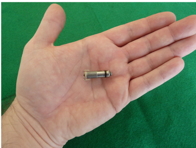
Fig. 1 The Micra ® TPS LP system is currently the only available leadless pacing system. The first implantation in a human patient was performed in December 2013 in Linz, Austria
