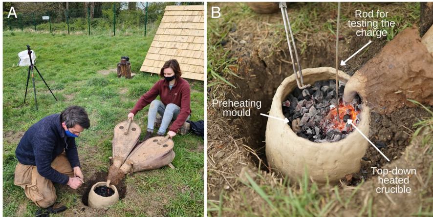
Fig. 15 A Photo of B. O'Neill and L.E.F. Brown in the field during the experiments at UCD CEAMC using bellows to pump air into the cylindrical furnace. B Close-up photo of the furnace structure with charcoal and an experimental crucible charged with copper and tin. The area directly heated by the bellows' nozzle is the hotspot, which reaches highest temperatures
