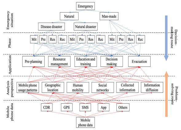
Fig. 4 Framework of using mobile phone data for EM. Note: Mit = Mitigation; Pre = Preparedness; Res = Response; and Rec = Recovery
