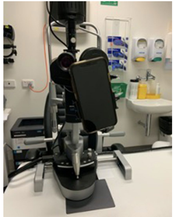
Fig. 2 Set-up of the slit lamp adaptor on the Haag-Streit BQ-900 slit-lamp using an iPhone 11 (Apple, Inc., Cupertino, Calif., USA)
