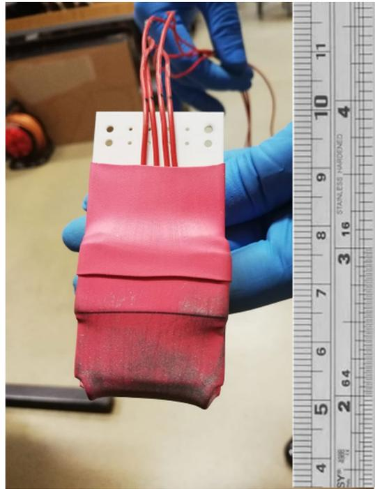
shrinking properties. The material details are not disclosed by the company, just irradiated cross-linked modified polyolefin. On shrinking the tube, we tried to avoid bubbles staying inside the sensor.
