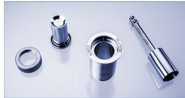
(b) High pressure set up in Double Gap geometry
