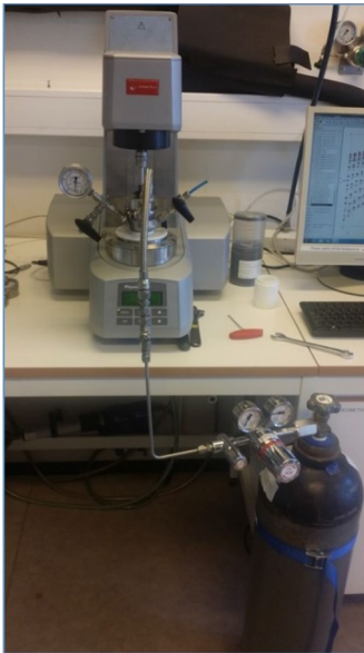
(a) Anton Paar MCR 301 Rheometer with the connected nitrogen tank used for running the experiment
