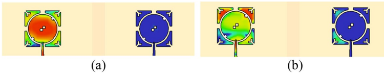
Fig. 52 Surface current distribution over the patches of the side-by-side MIMO antenna system at (a) 28 GHz and (b) 38 GHz
