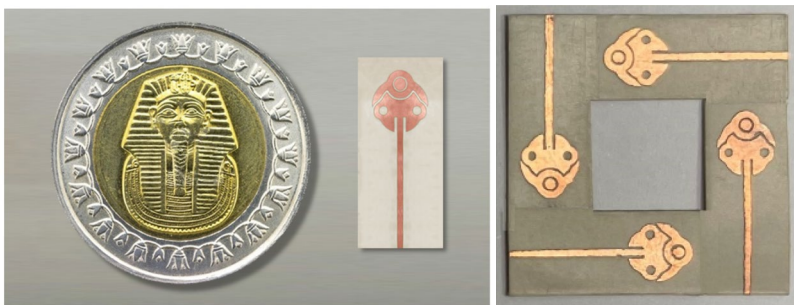
(a) The fabricated model of the dual-band antenna, (b) Fabricated MIMO antenna system.
