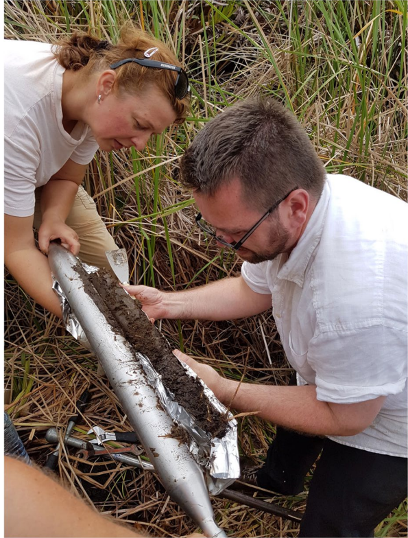
Fig. 2 Examining a core taken with a Russian Corer in Point D'Esny, Mauritius. Photograph by Krish Seetah
