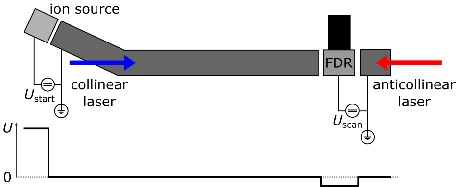
Fig. 1 Simplified scheme of collinear laser spectroscopy. Electrostatically accelerated ions are superposed with a copropagating or counterpropagating laser beam. Fluorescence light is detected with a photo multiplier tube in a floatable fluorescence detection region (FDR). Doppler tuning is performed by changing the voltage at the FDR as indicated
