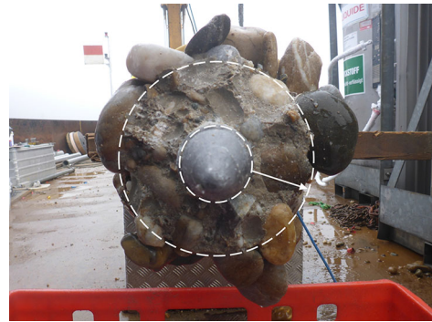
Fig. 4 Freeze core sample—cross section. The interrupted lines show the extent of the sampling space
