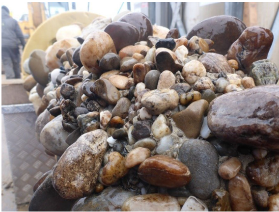
Fig. 3 Freeze core sample—close up
