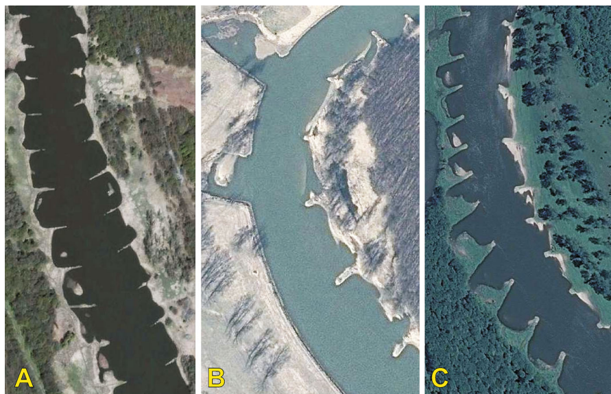
Fig. 1 Examples of groyne distribution in the Oder valley: A groynes of similar length on a straight stretch of the river; B irregularly shaped groynes along one of the river banks; C groynes of different lengths on both banks of a river bend (source: Google Earth maps)
