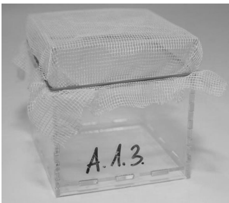
Fig. 1 An example of an experimental Plexiglas cube used in Experiment 1 to study the aggregation and attachment of zebra mussels. Each box consisted of five detachable walls (70 × 70 mm) and was covered with a square piece of mesh held in place with a rubber band to prevent the mussels from escaping
