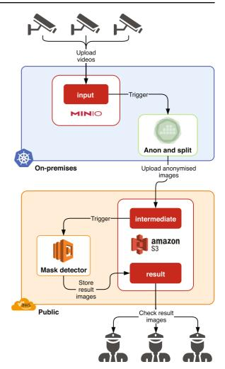
Fig. 4 Workflow for the defined use case involving face mask detection on anonymised images on a hybrid Cloud
