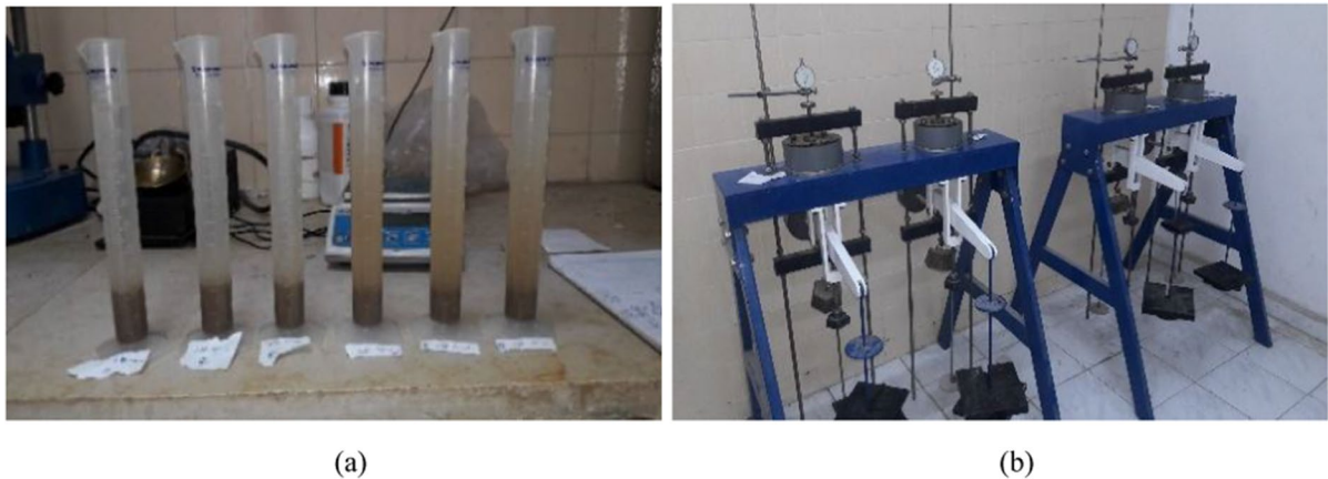
Fig. 3 Free swelling (a) and Confined swelling (b) experiments of different percentages of added sand
