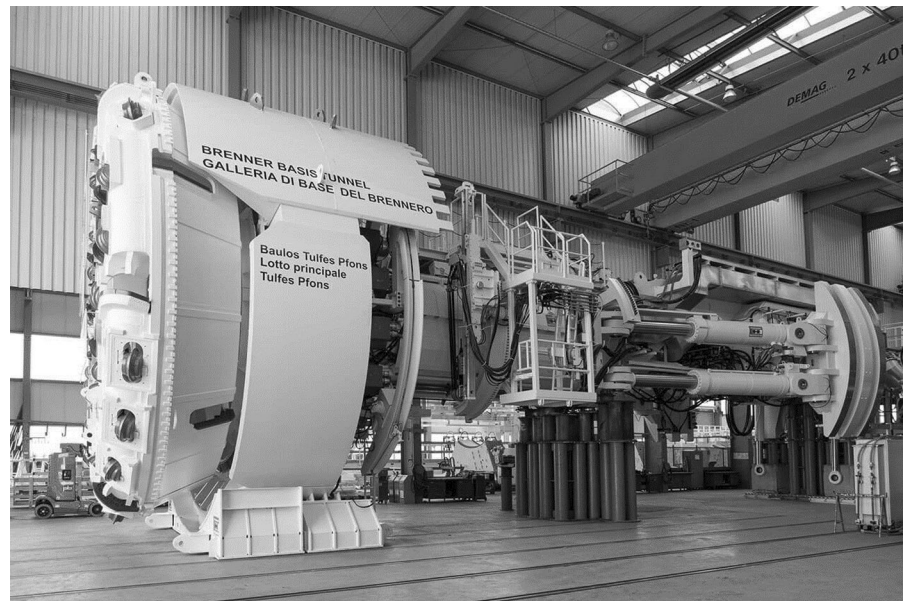
Fig. 2 Side view on the gripper TBM used during construction of the exploratory tunnel Ahrental-Pfons. (“bbtinfo.eu,” 2020)
