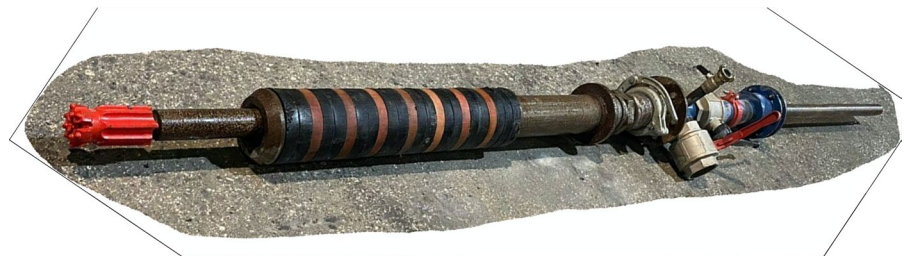
Fig. 8 Innovative standpipe-packer with attached preventer and threaded tube drill pipe
