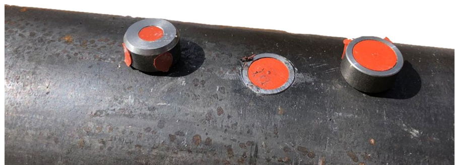
Fig. 7 Grouting inserts (self-sealable valves) installed in a grouting pipe (middle) and removed grouting inserts (bottom of the valve, left/top of the valve, right)
