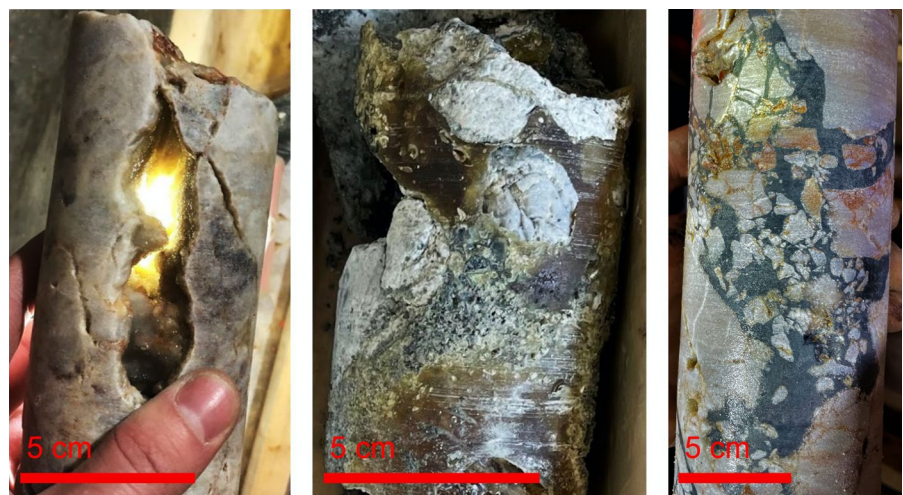
Fig. 3 Drilling core of Grasberg-limestone with karst (left), drilling core from weakness zone of Otter-dolomite with polyurethane grout (middle), and a sample of a carbonatic breccia from the transition zone with cement grout (right)
