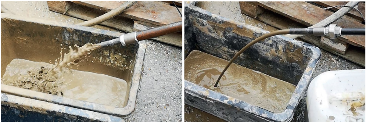
Fig. 11 Comparison of standard cement grout mixes (left) and combined cement-polyurethane grout mixes (right)
