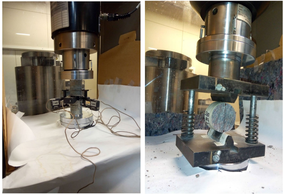
(a) Rock specimen held by extensometers for uniaxial compression testing
