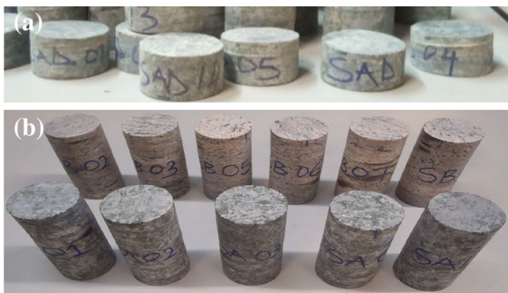
Fig. 3 Core samples of rock for a Brazilian tensile strength tests, b uniaxial compression tests
