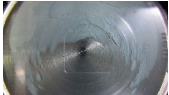
Fig. 1 Effect of stress whitening in DOWSIL™ TSSA under volumetric loading during experiments
