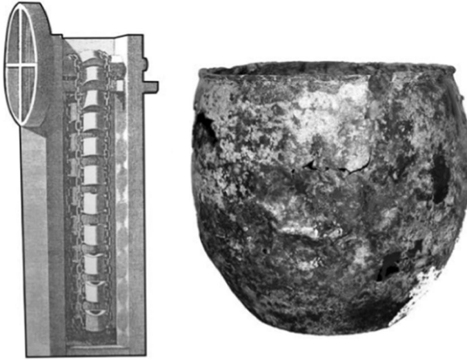
Fig. 9 Left, Illustration of a bucket pulley. Right, Roman bronze bucket preserved in the Mining Museum (Huelva) (Arboledas-Martínez, 2013)
