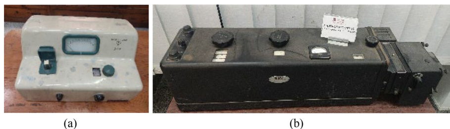
Fig. 14 Two models of spectrophotometers: a A “ Spectronic 20 ” spectrophotometer (only visible), Bausch & Lomb, 1955; b A UV–visible spectrophotometer, introduced by Beckman in 1941 and made by the National Technical Laboratories of South Pasadena, CA. Both instruments are at “Primo Levi Museum”, “La Sapienza University” of Rome (Italy)
