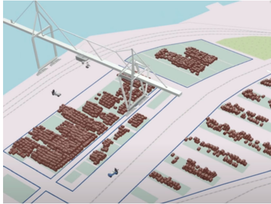
Fig. 5 Digital twin visualization at the Weserport (provided by OHB, systems provider based in Bremen)
