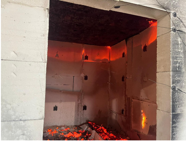
Figure 14. Flaming behind plasterboard and in cracks in boards for partially protected solution.
