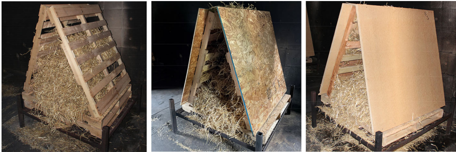
Figure 2. Fuel loads for replicate experiments with (left) pallets and straw, (center) OSB, pallets and straw, and (right) fiberboard, pallets and straw.
