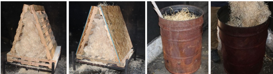
Figure 3. Fuel loads for exploratory experiments with (from left to right) pallets and excelsior; OSB, pallets and excelsior; smoke barrel with wetted straw; and smoke barrel with wetted excelsior.
